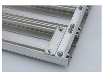
end. Repeat for all legs. To attach these legs, slide  $\frac{1}{4}$ -20 X  $\frac{1}{2}$ " hex bolts into the mounting slots at the four corners of each track section and one additional bolt into the slot next to that one. Place the stabilizer bracket on these two bolts and tighten a nut only on the one bolt as shown in the picture.
